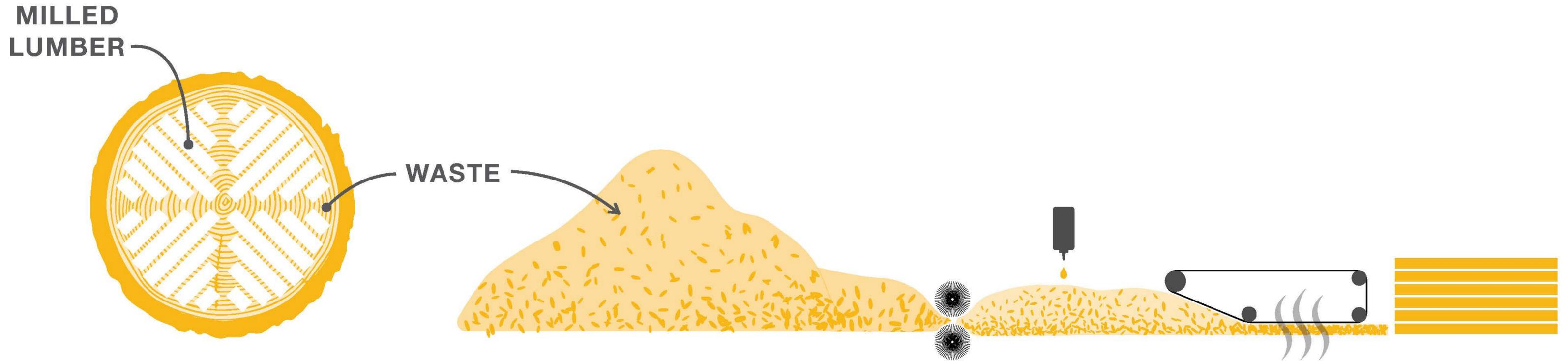
LUMBER IS MILLED FROM LOGS. THE WASTE CHIPS & SAWDUST IS RECOVERED, FINELY GROUND, AND FORMED INTO INSULATION
